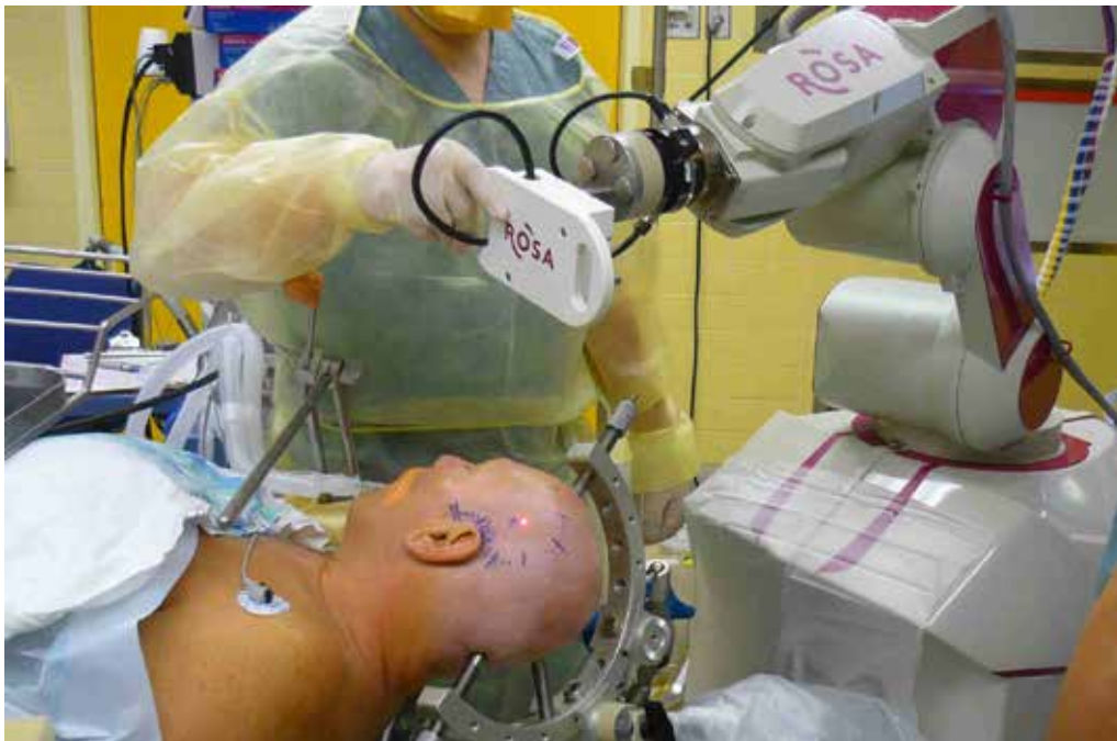
Fig.21 Use of robot for topographic and functional guidance in craniotomies
