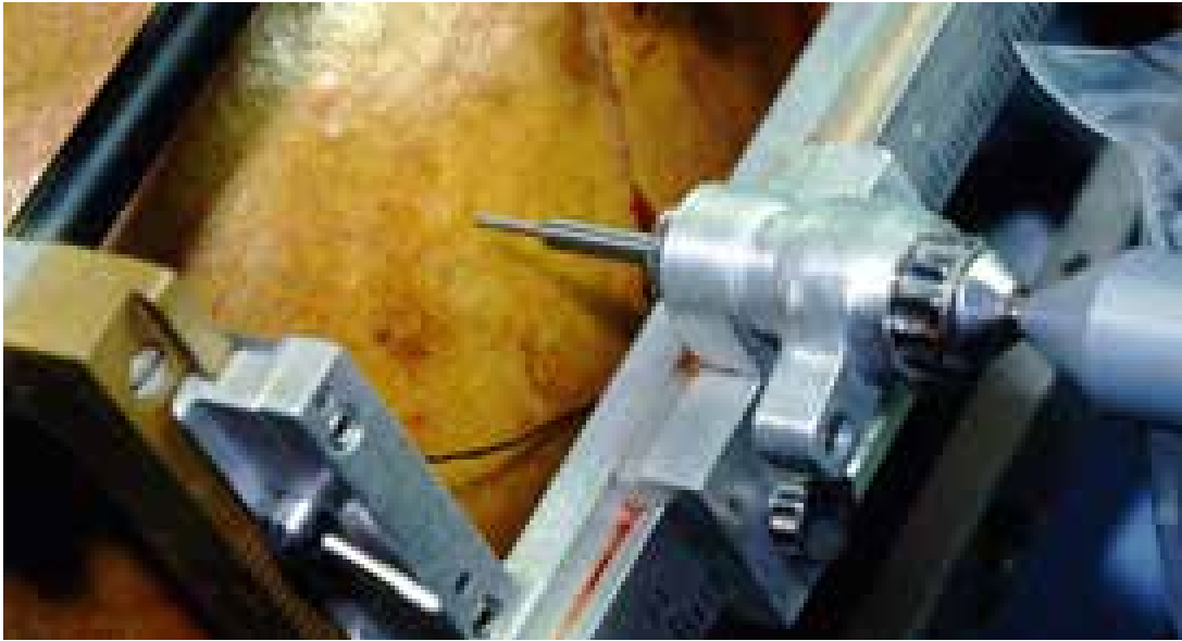
Fig.7A Orthogonal Carrier to insert depth electrodes
