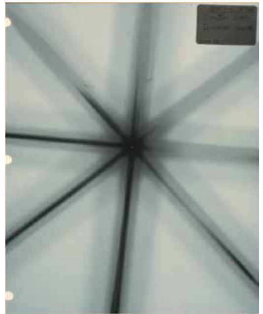
Fig. 17b Photon beams generated by linear accelerator
